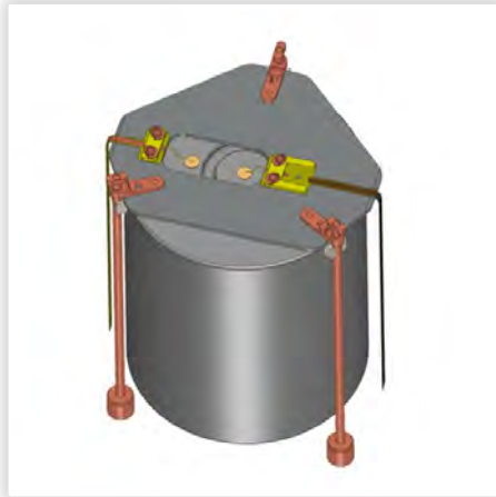
Inverted coaxial point contact Ge detector 300–400 detectors at ~3 kg each
